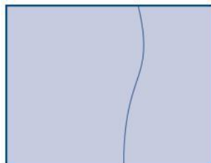
Fig. 29 Twist cracking in a glass unit.
