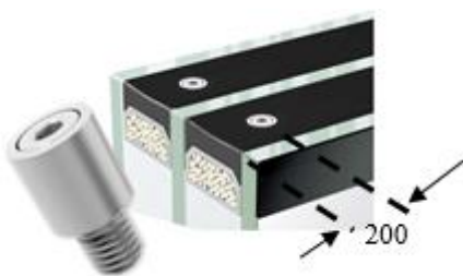
Fig. 27. Open type valve of the Swisspacer spacer.
